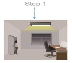
The sensor switches on the light automatically when person enters the room
